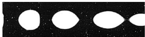
Fig. 8. Natural jet at Re = 180 , Fr = 1.0 , fluid combination 2. Length of each image is 13.5 D
