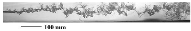
Fig. 3 Dye visualization image for Re = 10,000 and D = 4.7 \text{ mm} . The flow direction is left to right
