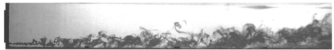
Fig. 3. Side view of a plume released isokinetically 25 mm (0.125H) above the bed into a fully developed turbulent boundary layer in an open channel flow
