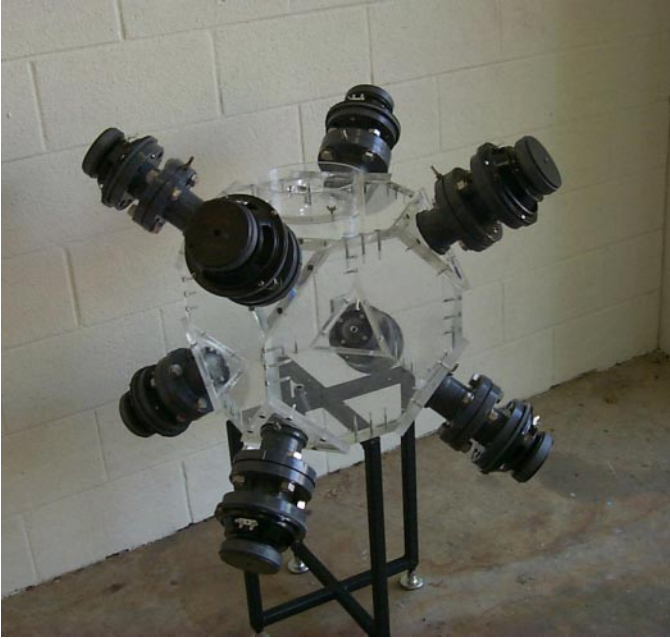
Fig. 2. Photograph of the turbulence chamber and actuators
